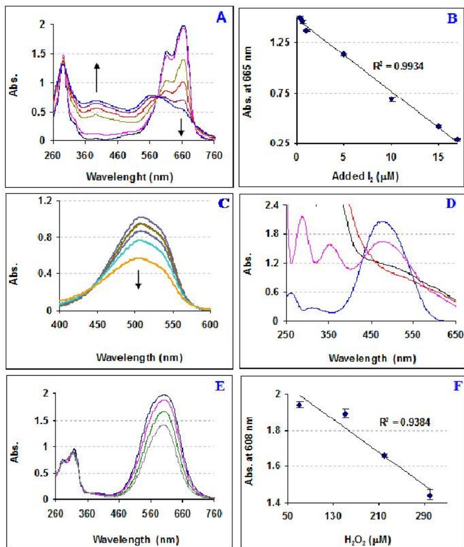
**Fig. 4.** Overlaid spectra of the reaction mixture of iodine solution with **A)** MeB and **D)** MADA. Overlaid spectra of the direct reaction of  $\text{H}_2\text{O}_2$  with **C)** MO in the presence of Fe(II) at room temperature and **E)** MB at boiling temperature. Changes in the optical density of **B)** MeB at 665 nm at room temperature and **F)** MB at 608 nm at boiling temperature. Reactions were carried out at pH(s) summarized in Table 1.
