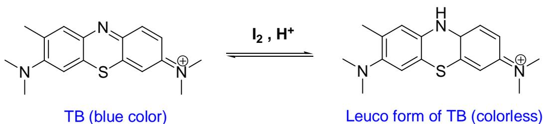
**Fig. 1.** Discoloration of TB in the presence of iodine in acetate buffer (2 M, pH 8).
