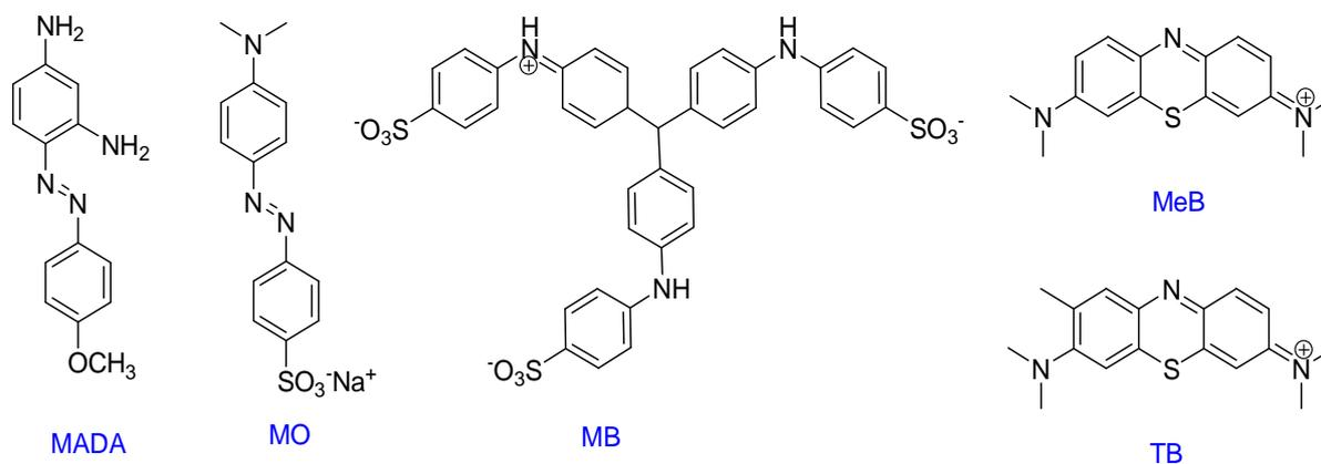
**Fig. 2.** Chemical structures of the organic dyes employed in the spectrophotometric studies of this research.
