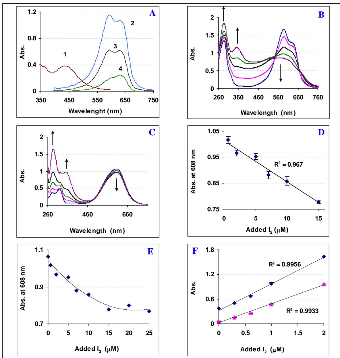
**Fig. 3.** UV-Visible spectra of **A)** acidic iodine solution (1) and TB at three different concentrations (2, 3, and 4) in acetate buffer (2 M, pH 8). Overlaid spectra of the reaction mixture of iodine solution with **B)** TB, **C)** MB. Changes in the optical density of **D, E)** MB at 608 nm, and **F)** MB at [■] 290 and [▲] 360 nm solutions after successive addition of iodine at room temperature. Reactions were carried out at pH(s) summarized in Table 1.
