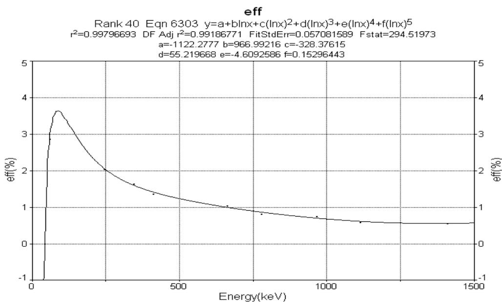
**Fig. 2.** HPGe detector efficiency versus gamma photon energy. The calibration curve has been shown as solid line. Squared points represent measured data.
