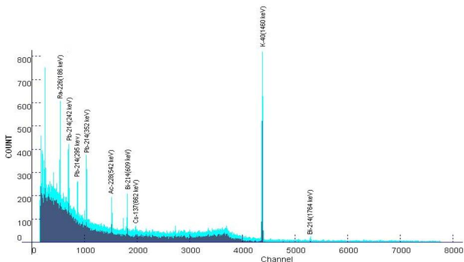
**Fig. 3.** Measured gamma spectrum for CAFC sample in Marinelli flask. Given energies in blankets are in units of keV.
